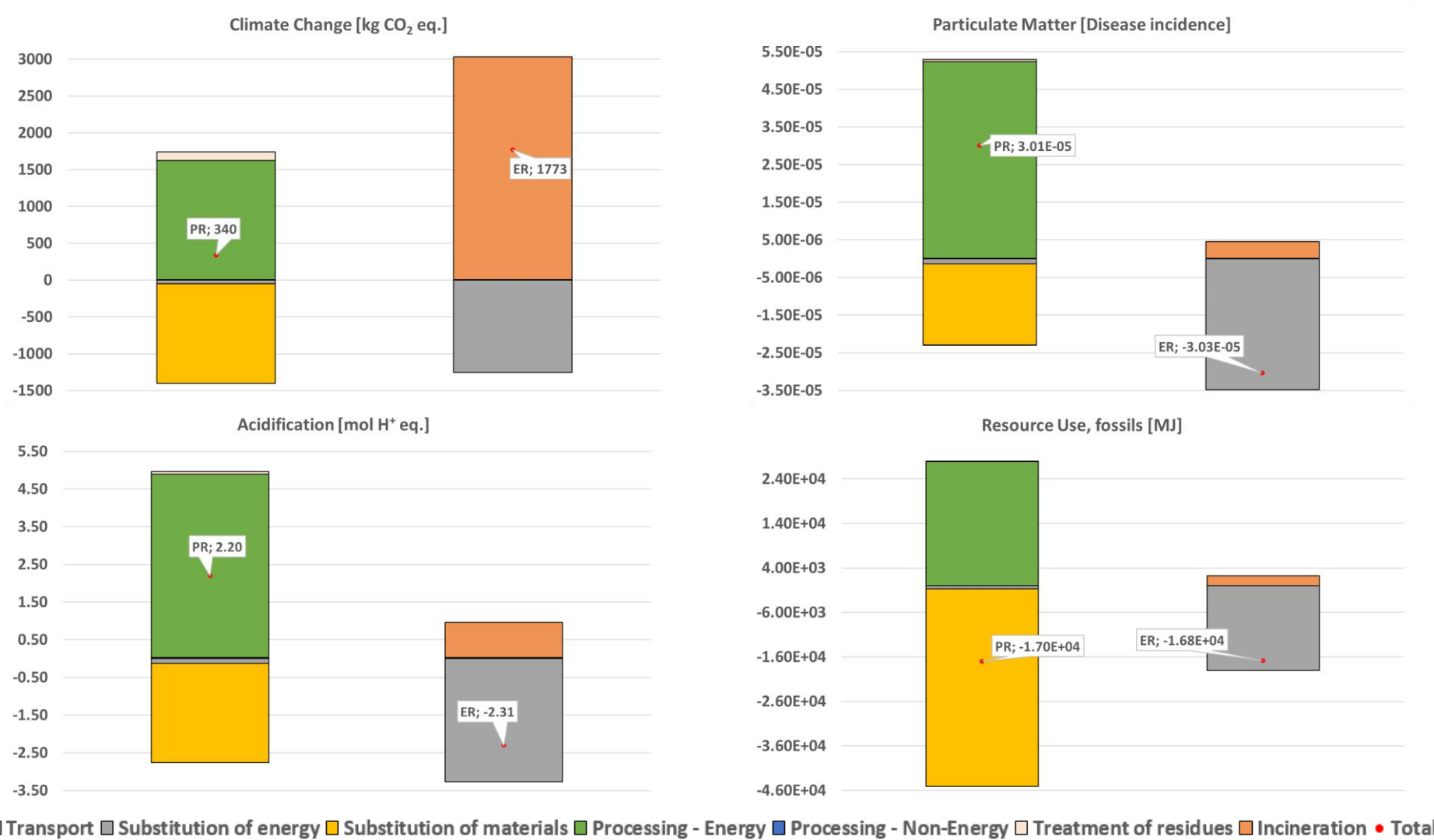
Figure 9. Management of 1 tonne of EPS construction and demolition waste through physical recycling (PR: solvent-based separation/dissolution and subsequent PS granulate production) and energy recovery (ER: incineration): Climate Change, Particulate Matter, Acidification, and Resource Use, fossils impact indicators. Negative values represent savings, while positive ones represent burdens. See Table 1 for a description of the different treatment scenarios and technologies.
